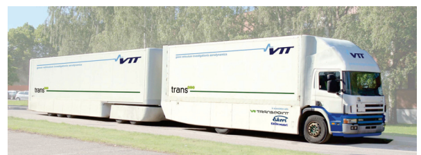
Figure 4: Test vehicle with the aerodynamic upgrade kit.
