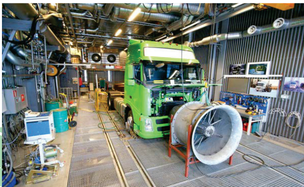
Figure 2: Chassis dynamometer facility at VTT allowing heavy vehicles to be tested up to 60 tonnes of GVW.
